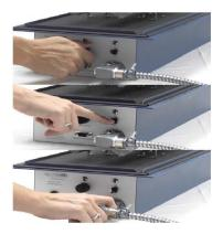
6. Carefully remove the tube from the unit by first pulling the end cap screw out of the L-bracket, then by sliding the tube out of the loosened clamp.
